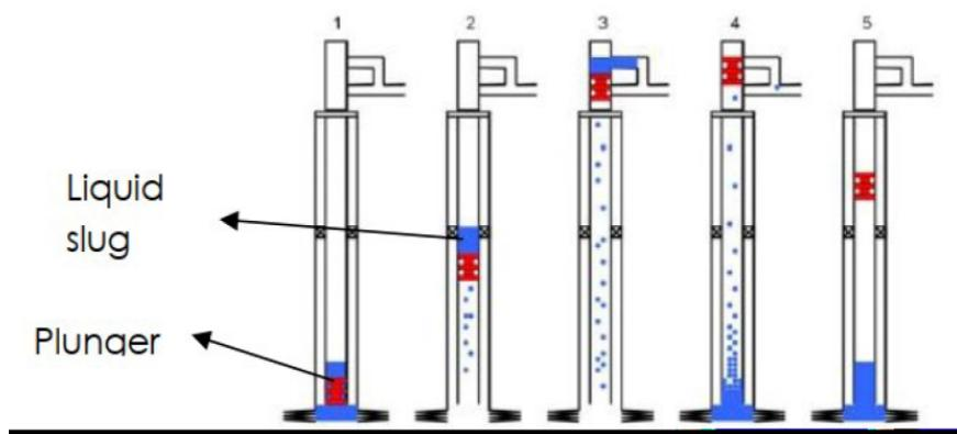
Figure 2. Schematic Operation of Plunger Lift (Gasbarri & Wiggins, 2001)
