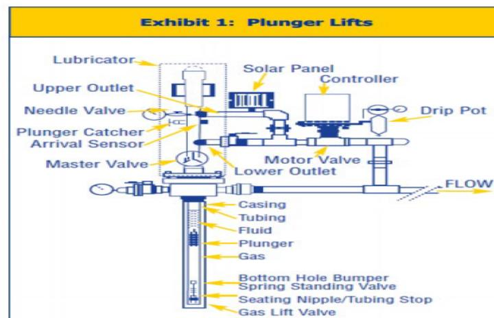
Figure 1. Installing a plunger lift on a gas well (Gasbarri, 1996)
