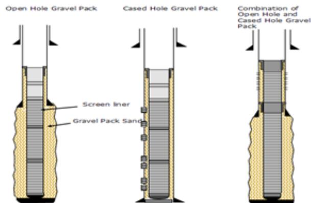
Figure 7. Open Hole, Cased Hole, and Gravel Pack Combination
