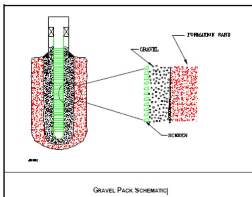
Figure 6. Schematic Gravel Pack and Slotted Screen (Penberthy Jr & Shaughnessy, 1992)
