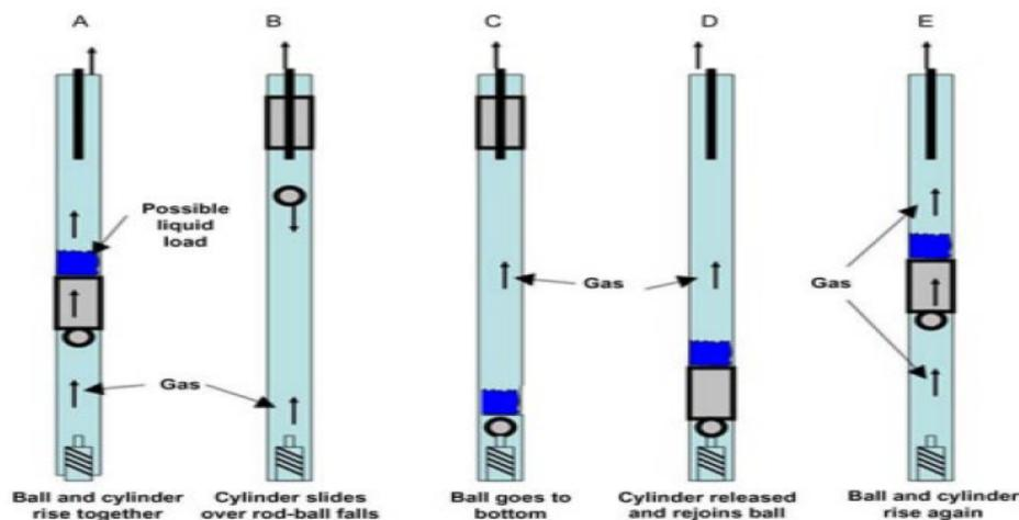
Figure 3 Continuous Plunger Cycle (Gasbarri & Wiggins, 2001)
