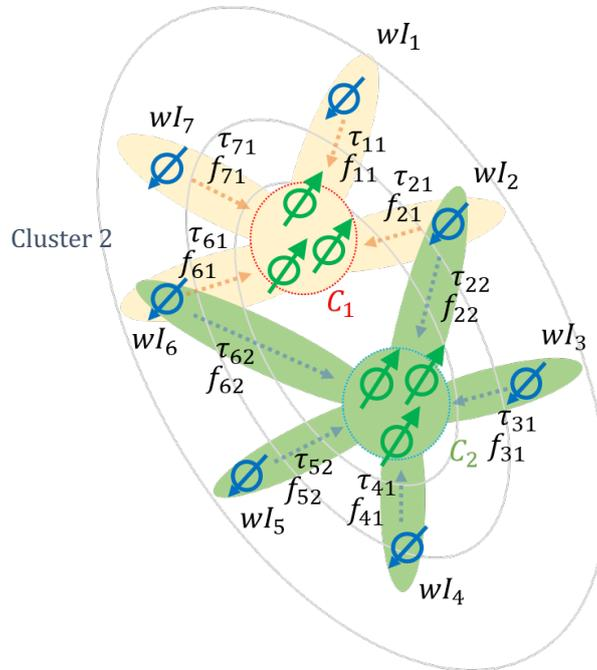
Figure 2 Illustration of injector-clustered producer pair-based control volume, CRM-IPC. Control volumes originating from the injector are permutated to all production well clusters. Grey lines represent contour depth for a typical anticline structure.
