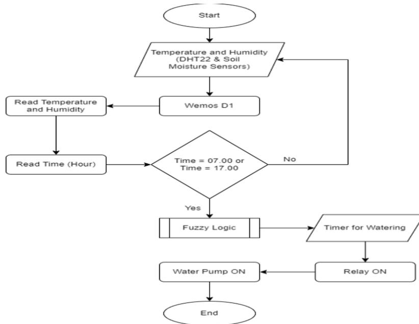
Figure 3 . System Workflow
