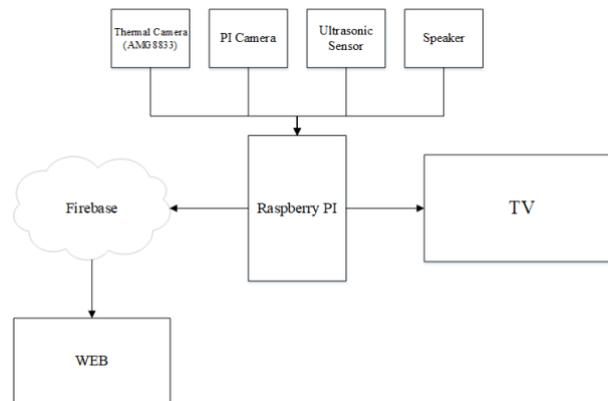
Figure 5. Tool architecture
