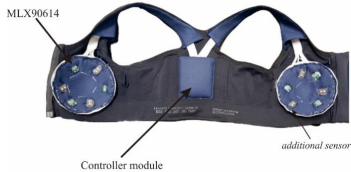
Figure 5. Installation of the MLX90614 sensor on the bra cup and the controller module board on the back of the bra
