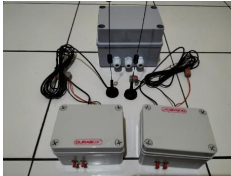
Figure 5. LoRa Node and LoRa Gateway tools
