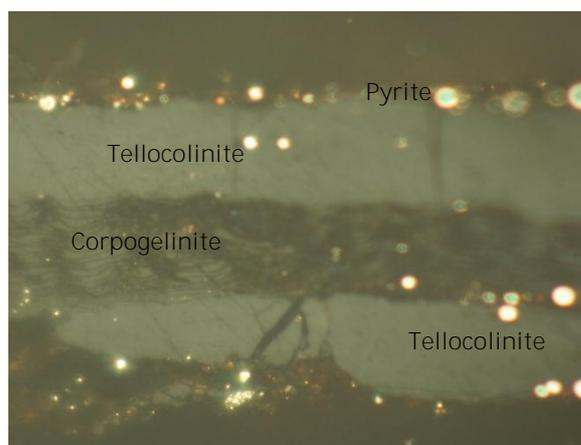
Fig 4. Corpogelinite and pyrite associated with desmocollinite in coal, reflectant white light, 500x. Sample 6103/16.
